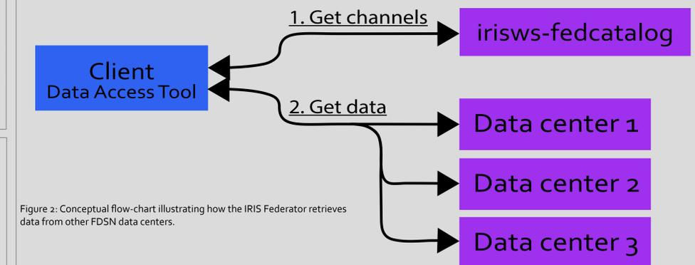
Figure 2: Conceptual flow-chart illustrating how the IRIS Federator retrieves data from other FDSN data centers.
